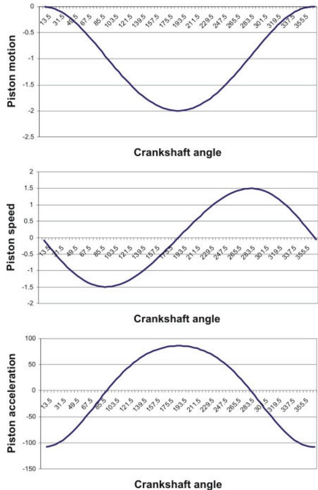
Figure 8. Simulation of single cylinder motor's kinematics [05]
