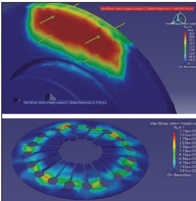
Figure 7. Stress analysis of a rotating brake disk and diaphragm clutch spring
