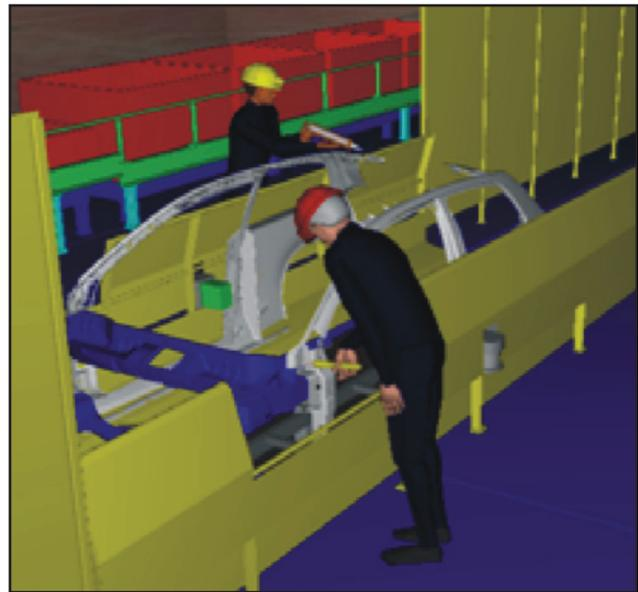
Figure 16. Ergonomic optimization of a body welding work cell [03]
